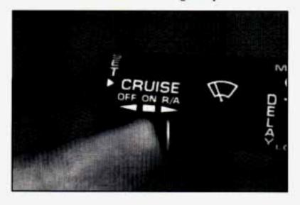
Move the cruise switch from ON to R/A (Resume/Accelerate). Hold it there until you get up to the speed you want, and then release the switch.
